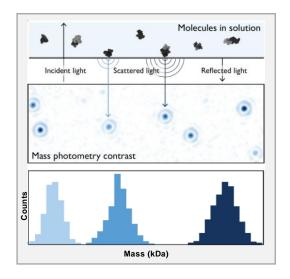
Mass photometry measurements provide the mass distribution and relative concentrations of a wide range of biomolecules in a sample. The method is suitable for sample **purity** and **homogeneity**, **protein oligomerization**, **biomolecular interactions** and **macromolecular complex assembly** determination.
